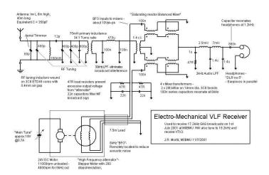
It is basically a direct conversion receiver. It has a 2 pole passive preselector with a RF bandwidth of about 800 Hz, which also impedance matches the antenna to the mixer. The mixer uses saturating ferrite cores, in a way not unlike the SAQ keying circuit. The BFO signal saturates the cores at both the positive and negative peaks of it's waveform, and so the core windings present an inductance that varies at twice the BFO frequency, in series with the signal path.
